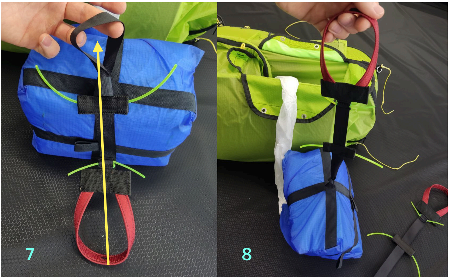
7,8) Connect the rescue handle to the parachute envelope using a choke knot.
