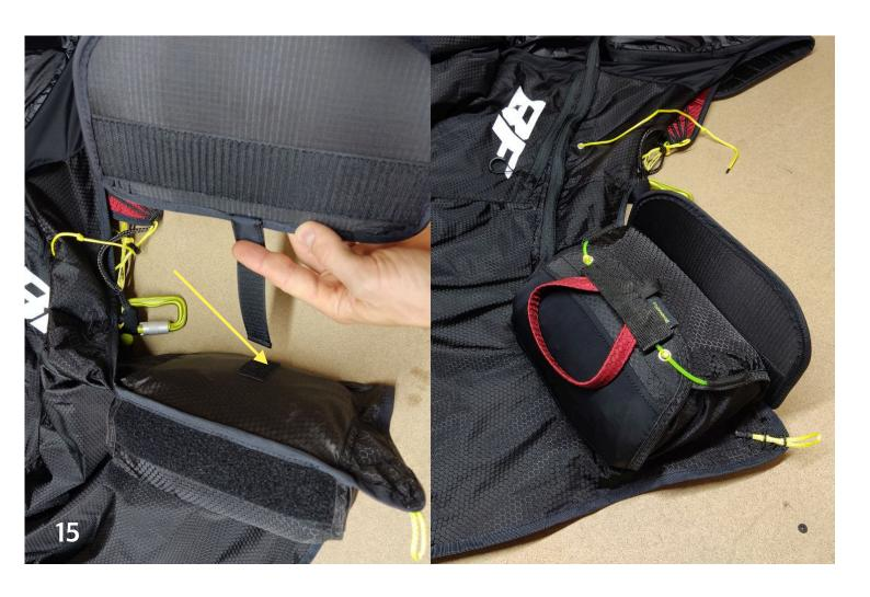
**15)** Attach the removable tool board. Use the tension of the Velcro tail to adjust its angle.
