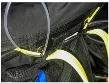
Close the reserve container flap using the two locking loops passed through the eyelets, and locked using the yellow cables on the reserve handle. The handle straps should be routed between the two locks.
