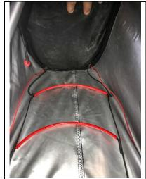
The lower two steps of the three step speed bar, showing bungee attachments to the base of the foot plate.
