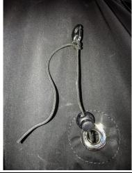
Cord-lock and Brummel hook on the Speed bar line where it exits the skirt through the eyelet.
