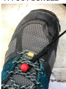
There is a bungee attached to the inside front of the pod footplate area, with a plastic ball at its loose end. Tuck the ball into the shoelaces of your shoe. This will aid hands free entry into the pod after take-off.
