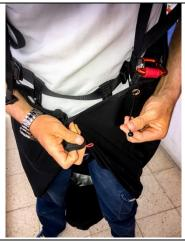
Locate the red loop on the right side of the pod closure, and match it with the plastic ball on the left side on the eyelet near the left carabiner.
