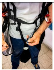
Next, locate the loop on the left side of the pod closure, and match it with the plastic ball on the pulley on the right, next to the carabiner.
