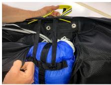
Place the reserve in the container with the handle attachments to the lower side as shown. In this way, the handle straps will help to open the zippers immediately. The reserve bridle should be under the reserve, and exiting into the zipped bridle sleeve, which can be closed later in the sequence.
