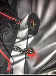
Left side ball bearing pulley and skirt eyelet with speed bar line in place.
