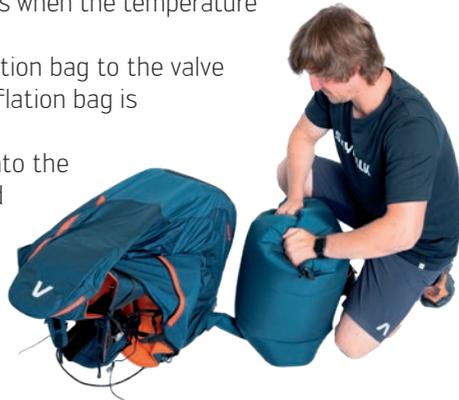
8. You will feel a pressure increase in the inflation bag when the protector is completely filled. It is not possible to pump more air into the protector. The check valve will ensure that no more air escapes.
