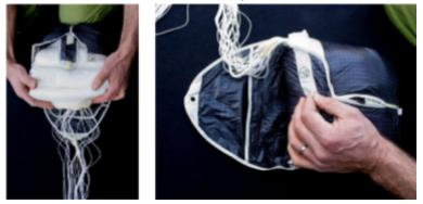
Close both sides of the inner container and the top pocket with the rubber, which you fix with one loop of all the suspension lines.
