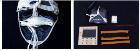
Use the last 20 cm of the suspension lines for the final closing of the inner container with the black rubber.
