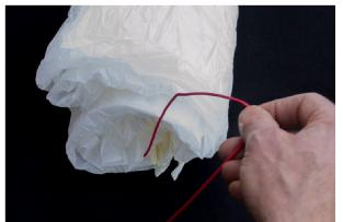
4.5 - S-folding canopy to fit into inner container (standard version)
