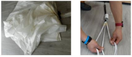
Check for the lines to run freely from the main riser loop connection to the canopy edge.
