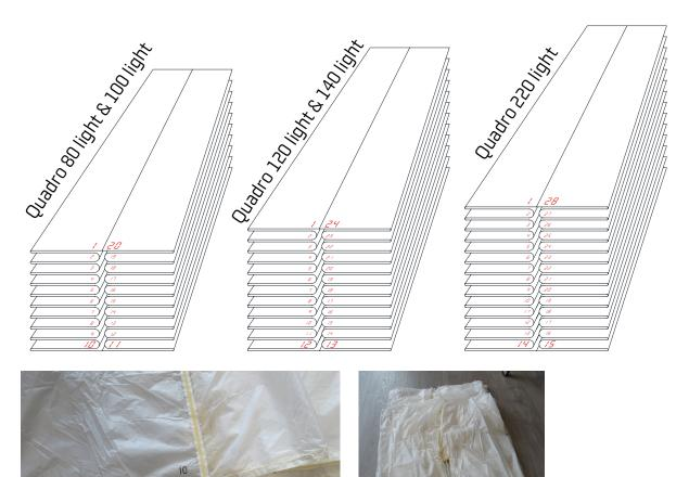
the canopy. Depending on the model the Quadro series have different numbers of packing loops attached to the canopy to enable an easy repack:
