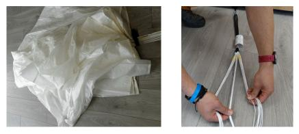
Check for the lines to run freely from the main riser loop connection to the canopy edge.
