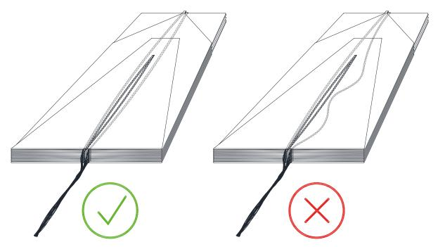
Take care that the internal edges between the panels are neat and properly tensioned.
