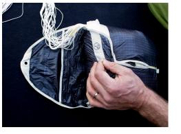
Close both sides of the inner container and the top pocket with the rubber, which you fix with one loop of all the suspension lines.
