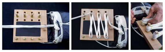
The suspension lines are sorted in three bundles, which are fixed by rubbers. These bundles are stored in the pocket of the container.
