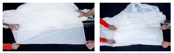
The last one is panel 1, which should be the top panel on the left side. Panels with slots are laid out as cone.
