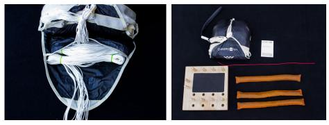
Use the last 20 cm of the suspension lines for the final closing of the inner container with the black rubber.
