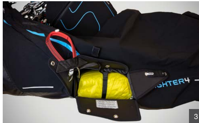
3 Insert the reserve with the handle attachment facing upwards and the lines underneath.
