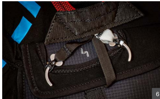
6 Insert the pins into their colour coded loops and pull the rubber pin retainer into position over the pin. Remove the threading lines!
