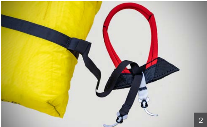
2 Connect the deployment handle to the side attachment loop using a larks foot knot.
