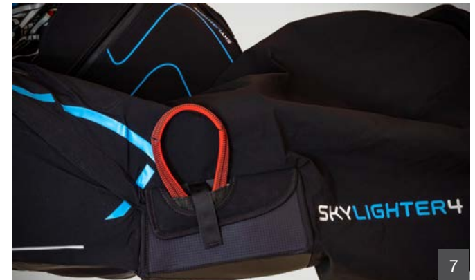
7 Position the pins and the handle underneath the neoprene cover. Secure the velcro tape and insert the final under surface leaf of the container into its pocket.
