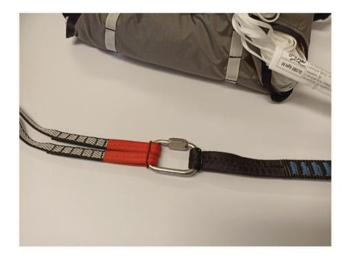
Secure the connection additionally with the neoprene cover supplied with the harness.
