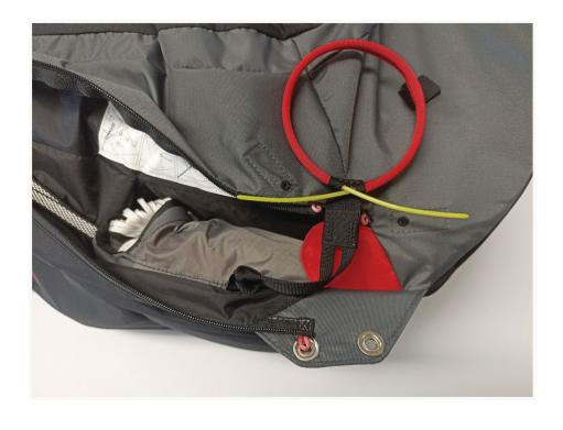
Using the auxiliary line, close the container following the sequence shown in the pictures.
