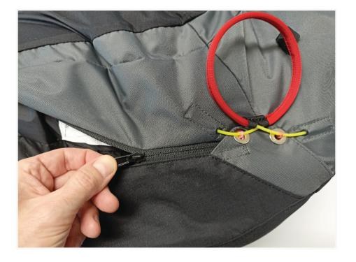
Caution: To avoid accidental opening of the rescue system, pins closing the container must be checked before each flight!
