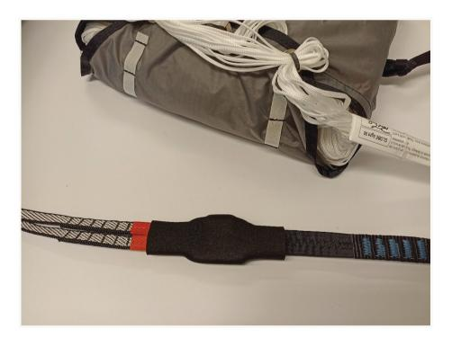
Lay the harness on its side and arrange the lines and v-riser in the container. Slide the rescue parachute into the container and attach the release handle with Velcro.
