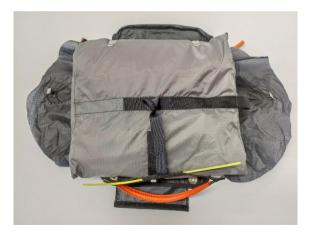
Pass the assistant lines through the loops in the No. 1 flaps. Then proceed as demonstrated in the pictures. Use temporary pins. The flaps of the container are marked with numbers 1, 2, 3. Close them in that order.
