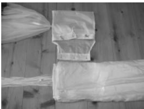
13. place inner container aside folded basis
