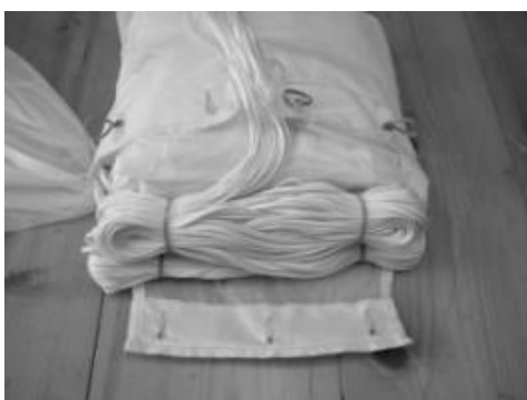
22. place line bundles close to canopy and guide the following lines through slit of containe
