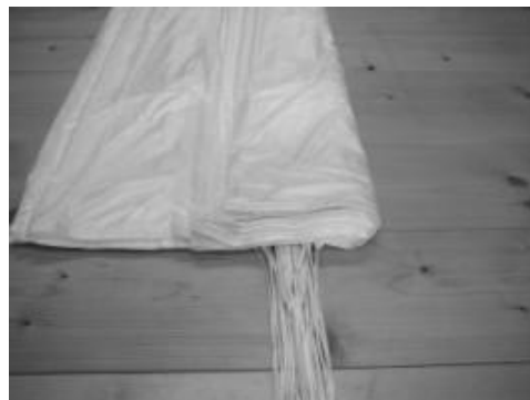
10. fold canopy into thirds, first on one side ..
