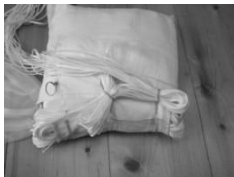
24. close right side of flap same way and make a line loop through rubber ring
