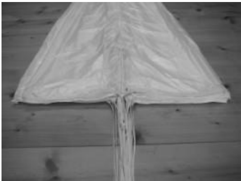
5. fold panels left and right same amount (each 12), with panel number 1 up
