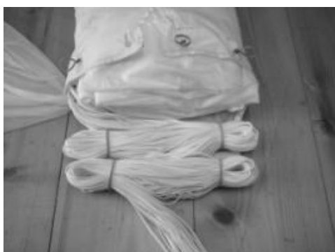
21. place rubber rings over ends of 8-bundles
