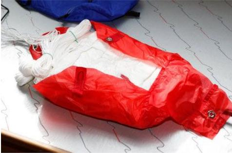
Carefully insert the cap into the cloverleaf container and remove the 3 packing cords
