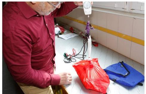
When lifting the reserve up by its lines, the closure must open under the its own weight
