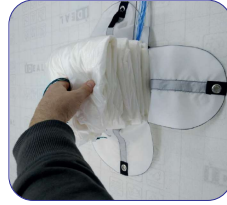
8. Put the layed canopy into inner container over the lines. Use for the canopy "snake" form folding method.
