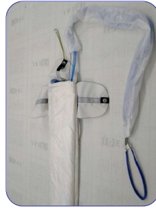
8. Put the layed canopy into inner container over the lines. Use for the canopy "snake" form folding method.
