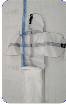
6. Lay the inner container under the lines near the parachute
