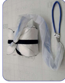
10. Close the folded canopy by all flaps of inner container. Secure the container by putting lines (lines together with cover) into black rubber loop.
