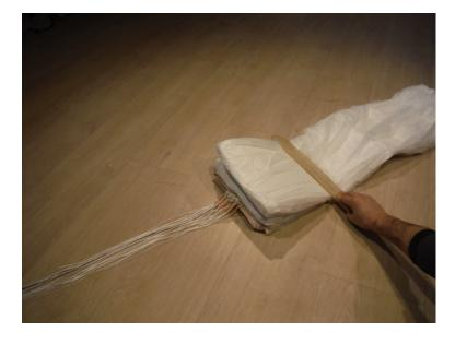
16. The canopy is now adjusted to width of the container with the s-flap
