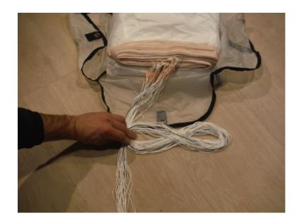
23. The P\_LIGHT should now be placed with narrow S-curves to a tower
