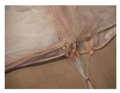
5. Sort canopy and it needs to be fix the lines with packing cord- lay panel 1 to the right
