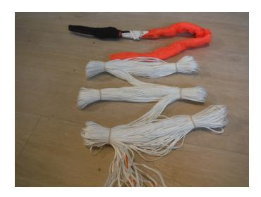
28. The line bundles are stowed away in the pocket of the line bag from the inner container. The P\_LIGHT Series should now be placed in S-curves. The length of the S-curves is depending on the size of the container. The length of the inner container from the P\_LIGHT-Series are different.
