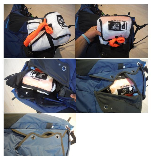
**PLEASE NOTE** \_ The riser of the P\_LIGHT should be connected to the suspension point of the harness. For the connection of the handle there are three loops on the outside face of the inner container.
