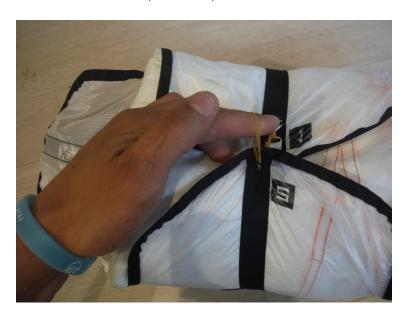
*32.* The cover sheet No. 4 of the inner container is closed with the plastic stick. The plastic stick is first pushed from the inside out through the small hole.
