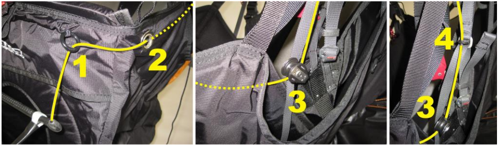
Fig. 21: Installing the speed system
