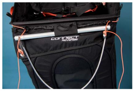
Fig. 6-18: Speed bar secured under the flap
