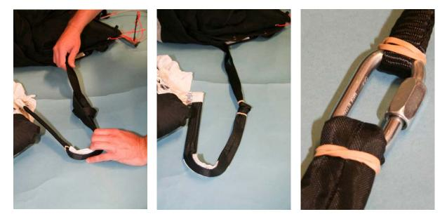
Fig. 5-3: Tighten the loops where attached
