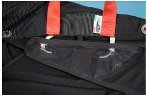
Fig. 5-18: Put in the ends of the deployment handle
