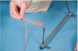
Fig. 6-17: Knot fastening the speed bar
