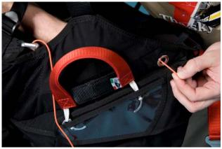
Fig. 6-14: Speed bar line through pulley
