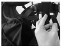
By adjusting the shoulder straps, the harness can be altered according to the height of the pilot. This is done using the adjustment straps integrated in the shoulder padding. During launch, the adjustment straps should not be tightened too much, because this will restrict your freedom of movement. A special holding system and elastic webbing hold the shoulder straps in place during launch.
