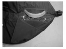
The deployment handle pins are then threaded through the elastic loops and underneath the transparent access cover. The pack cord must then be removed. Finally, the deployment handle is inserted under the cover incorporated in the harness
