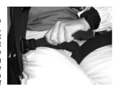
The adjustment is correct if you are able to get into your flying position without using your hands and if you have adequate freedom of movement for your launch run-up. Make sure that the leg loops are symmetrical.
