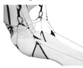
To increase the speed system travel, pass through only the lower ring: the speed bar pressure will increase.
