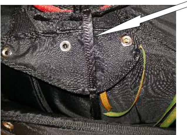
The connection to the handle runs between the two upper eyes. You have to take care that the connection of the handle is not hindered in any way and is still long enough, so that you can be sure that the pull is coming first on the closing-pins and not on the connection to the inner container!
