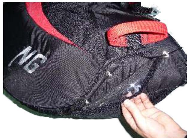
After closing the container, by putting in the pins, remove the packing cords and put the release-handle in the therefore assigned pockets
