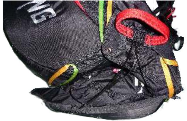
Put the bridle into the container of the harness. The connection to the handle must be also between the inner-container and the harness, as shown on the picture. That means it has to be on the inner side. So you can be sure that the rescue-system can be pulled out easily.
