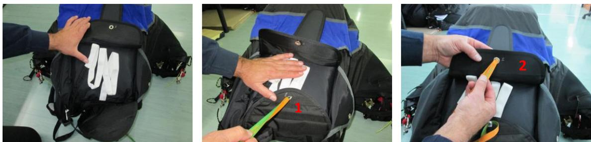
Take 2 pull up cords and close the rescue container covers as shown on the pictures below. At first close Top flap (1) with the bottom cover grommet (2) and after that the left side flap (3) and at the end the right side grommet (4).
