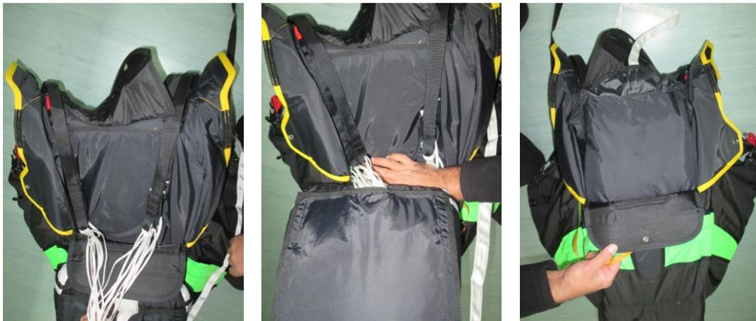
Fold the Rescue Static Line (RSL) on to the free bag.
