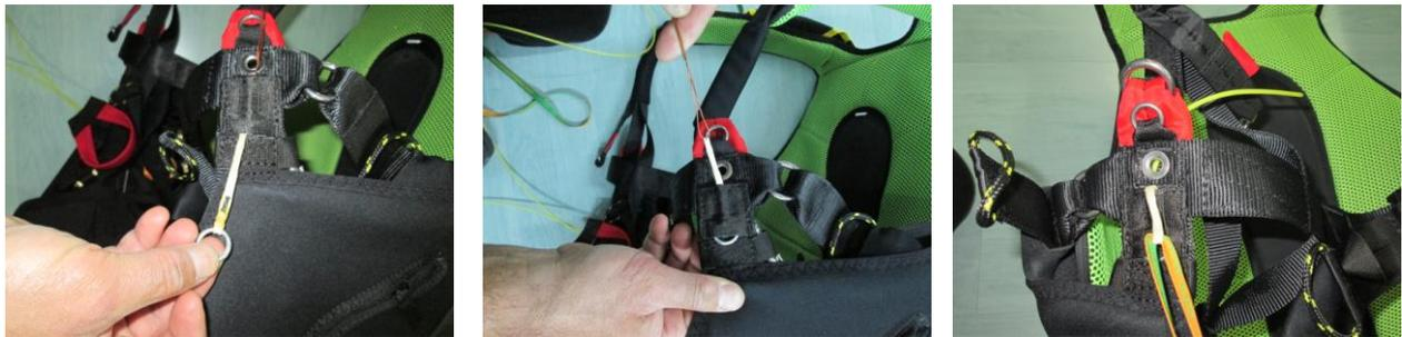
Pass the big ring trough the karabiner firs and after that the small ring trough the big one.
