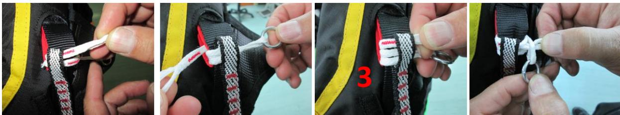
Wrap the soft link 3 times around the attachment point (3).
