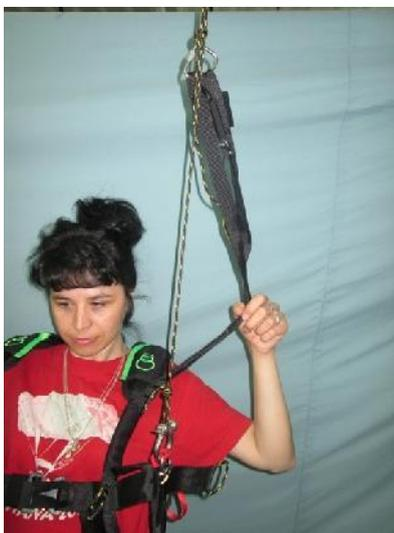
Attach the bottom end to the karabiners and at the top loop attach the rescue risers.
