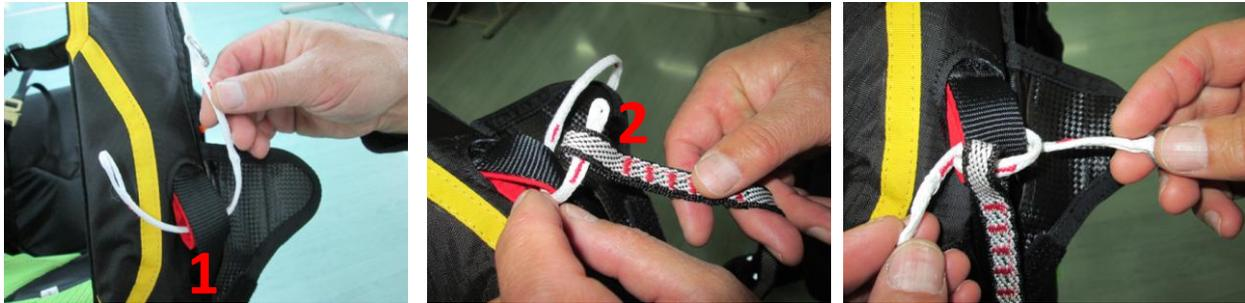
Insert the soft link line in the red attachment point (1) located at each shoulder belt ( under the magnets ), and the rescue attachment line (2).
