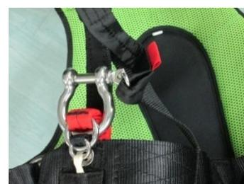
Attach the left riser of your wing to the left karabiner and tighten it. Make the same with the right wing riser and attach the RSL via Maillon Rapide® to the karabiner.
