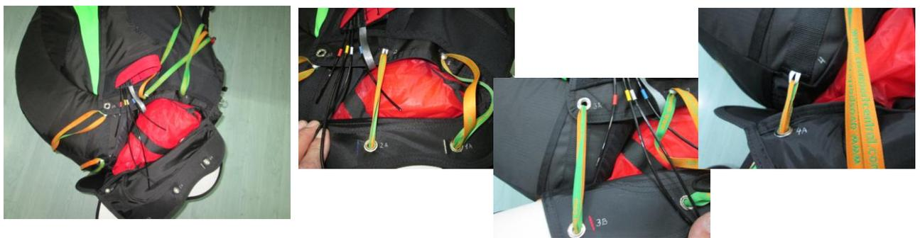
Pull the cord through the grommets and pin all the loops with the handles closing cable from 1 to 4. For your convenience there are different color markers on each cable and each grommet.
