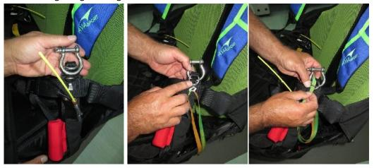
After that pass the packing line, from bottom to top, trough the loop, the small ring and the grommet.
