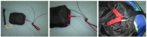
Put the rescue in to the harness container and using a packing line, close the container covers as sown on the pictures bellow. Don't forget to secure the loops with the black cables and at the end to remove the packing line.
