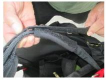
Attach the left riser of your paraglider to the left karabiner and tighten it. Make the same with the right paraglider riser and attach the RSL via Maillon Rapide<sup>®</sup> to the karabiner.
