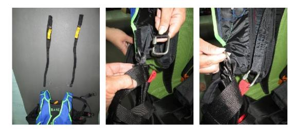
Use a packing line to pas it trough the loop. Pass the big ring trough the karabiner firs and after that the small ring trough the big one.
