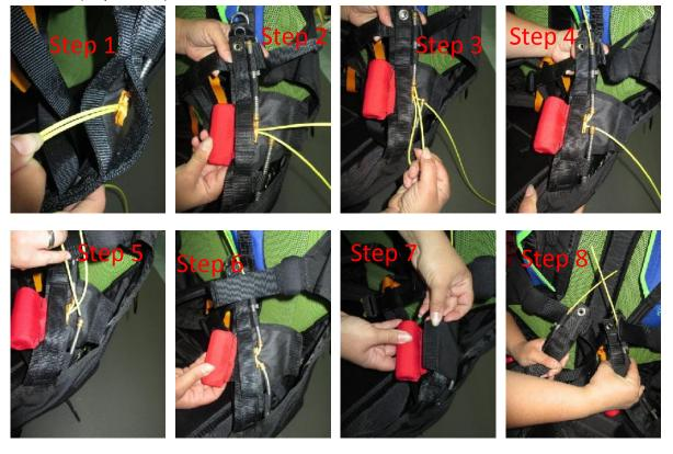
CHECK IF THE CUT AWAY CABLE IS PASSING TROUGH BOT HOSING
