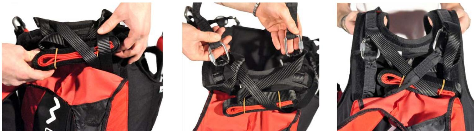
The two connections should be made using screw-lock karabiners with a breaking strength of at least 1,400 kg. In any case, it is important to verify that the length of the bridle is sufficient to position the reserve parachute inside the harness pocket, and that there is sufficient play to enable the parachute to be taken out of the pocket without causing the reserve parachute deployment bag itself to open during extraction.
