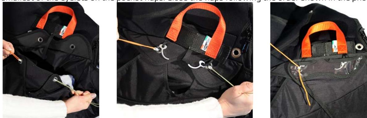
Push the metal pins on the handle into the elastic loops and under the transparent cover. It is essential to remove the cords after this operation. The cords should be pulled out slowly in order not to damage the elastic loops by excessive friction. Lastly, the handle should be positioned under the elastic cover.
