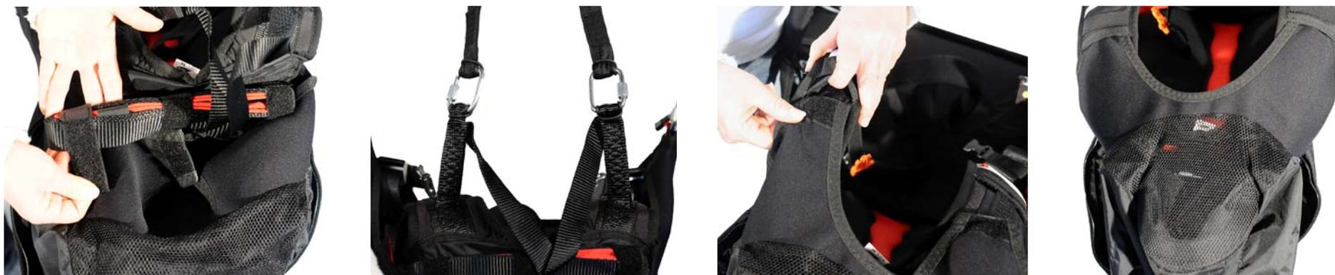
The two connections should be made using screw-lock karabiners with a breaking strength of at least 1,400 kg. In any case, it is important to verify that the length of the bridle is sufficient to position the reserve parachute inside the harness pocket, and that there is sufficient play to enable the parachute to be taken out of the pocket without causing the reserve parachute deployment bag itself to open during extraction.
