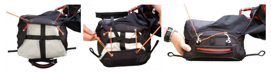
Inset the metal pins into the elastic loops, and insert the handle under the fabric flaps. The thin cord must be removed after completing this step. It should be drawn out slowly in order not to damage the elastic loops by excessive friction. Lastly, connect the right-hand loop of the emergency parachute bridle to the right-hand main karabiner.
