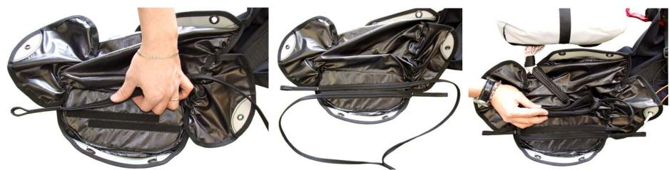
Insert the parachute into the harness container so that the deployment handle is visible and facing outwards, and with the loop that connects the handle to the deployment back facing upwards. Thread a thin cord (such as a paraglider shroud line) into each elastic loop. This will make it easier to close the container.
