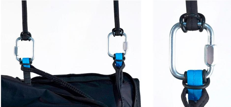
The two connections should be made using screw-lock karabiners with a breaking strength of at least 1,400 kg. It is important to verify that the length of the bridle is sufficient to position the reserve parachute inside the harness pocket, and that there is sufficient play to enable the parachute to be taken out of the pocket without causing the reserve parachute deployment bag itself to open during extraction.
