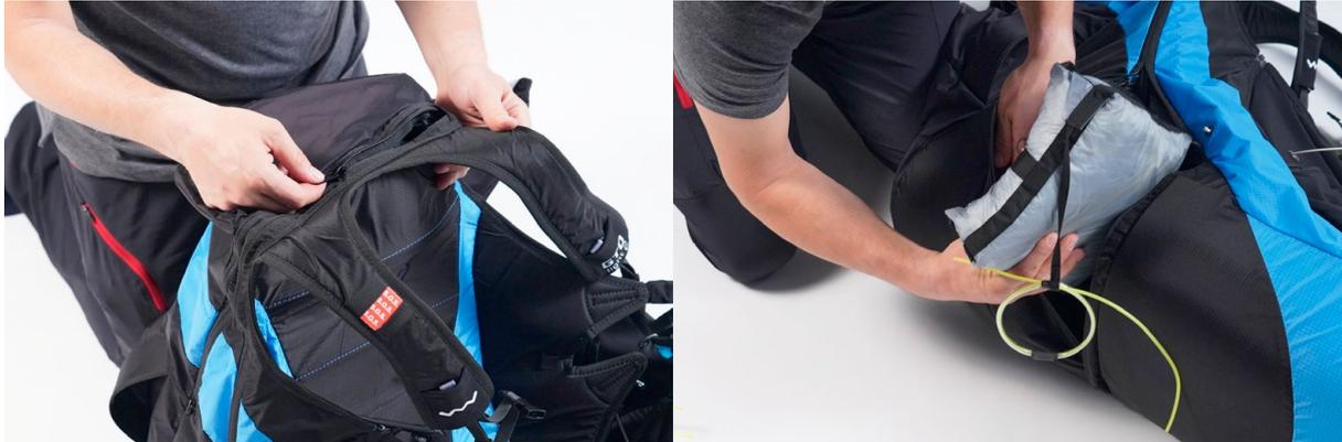
Insert the elastic loops in the corresponding pockets and through the small eyelets. Insert the parachute in the harness container with rescue handle facing upwards and rescue parachute lines facing the harness tail.
