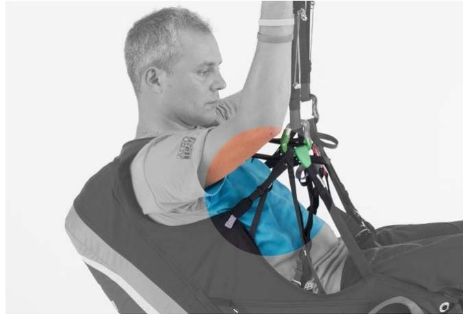
In this photo, you can see how the back adjustment works, dividing the load on two points per side for better comfort. This adjustment allows you to select the inclination of the torso with respect to the vertical flight axis.
