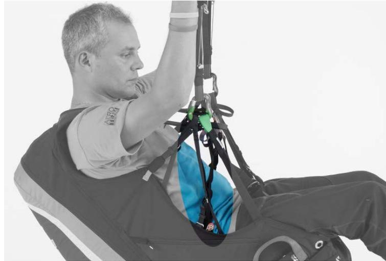
This adjustment varies the angle between the legs and the back (seating depth), distributing the load between the seat and the back, thereby providing the pilot with greater comfort. This adjustment is also divided into two points per side. If you want to change the adjustment, you must first loosen the strap as in the photos below.
