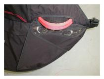
8 Fixing the safety cord: this particular type of cord (to be bought only from specialized dealers) must hold 5 kg. It prevents an accidental opening of your parachute. Using a needle, pass it through one of the holder's elastic loops and tie it to the pin (see photo).
