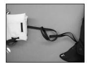
2 This connection may also be done using a karabiner – with a breaking load of at least 2000 kg. In this case the bridles must be fastened to the karabiner by means of elastics in order to avoid the karabiner from rotating on opening, which could bring about a dangerous lateral loading of the karabiner.
