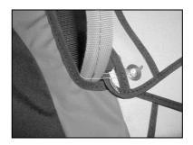
After the first assembly of your parachute you must perform an opening test and, before every take off, you must control the proper position of the handle.
