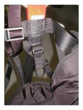
When adjusting the back, you must choose the torso inclination with respect to the vertical axis while flying. An excellent flying position for a better wing control can be obtained keeping the face about 15 cm from the ideal line that connects the two karabiners.
