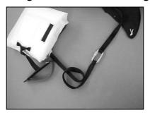
3 The karabiner's screw lock must be tightly screwed to prevent it from opening accidentally. This latter type of connection is more shock-absorbent than the conventional (former system) one.
