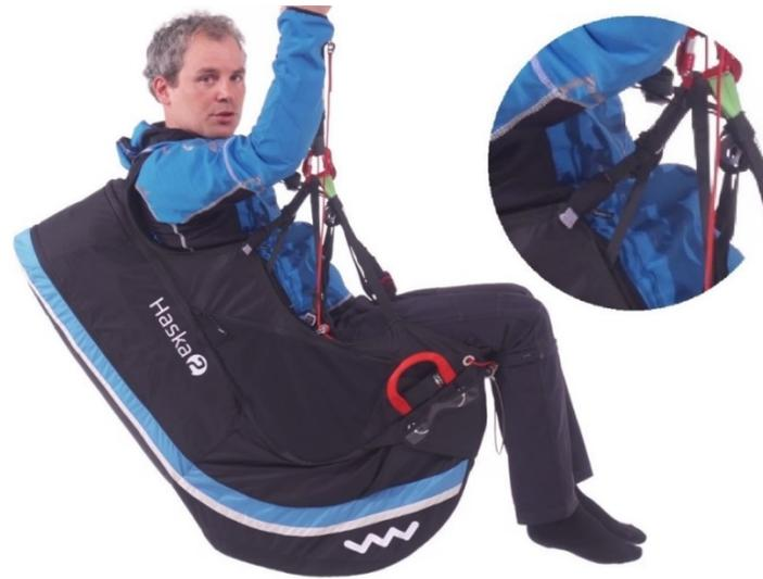
In this photo, you can see how the back adjustment works, dividing the load on two points per side for better comfort. This adjustment allows you to select the inclination of the torso with respect to the vertical flight axis.
