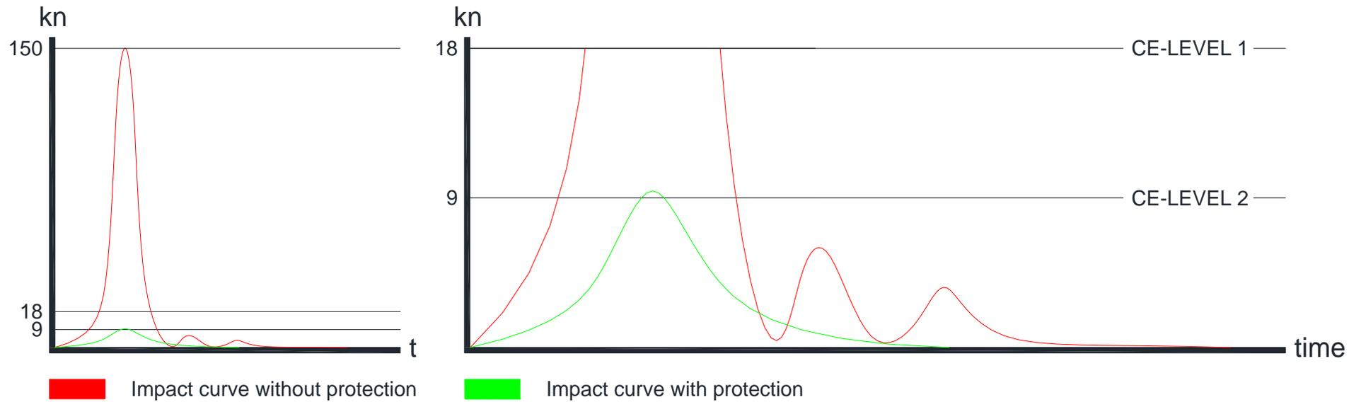
The shock absorbing properties of this back protection reaches the requested standard with a residual force of only 9,75 kN. This means that almost 94% of the impact gets absorbed by the back protection
