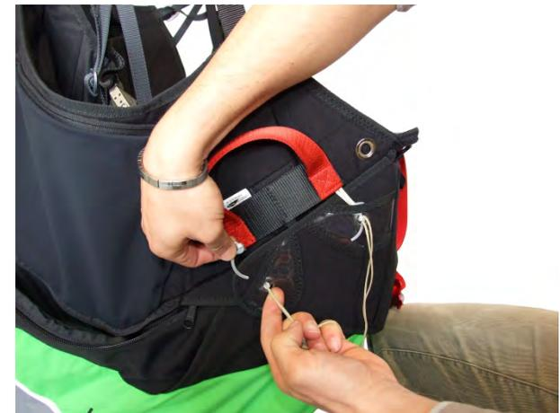
Introduce the handle's metallic pins into the elastic loops and under the transparent cover. The cord must absolutely be removed at the end of this phase, and must be extracted slowly in order to avoid damaging the elastic loops due to excessive friction between the parts. In the end the zip should be completely closed until introducing the zip pull under the cover behind the left shoulder-strap.
