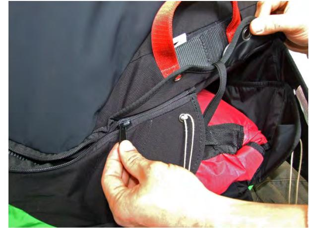
Take the bridle cover zip all the way to the right to then close it, moving the zip about 20 cm leftward. Then begin to close the various parachute container flaps, following the progressive order in the photographs, taking care during this phase that the zip does not open back up at the right end.
