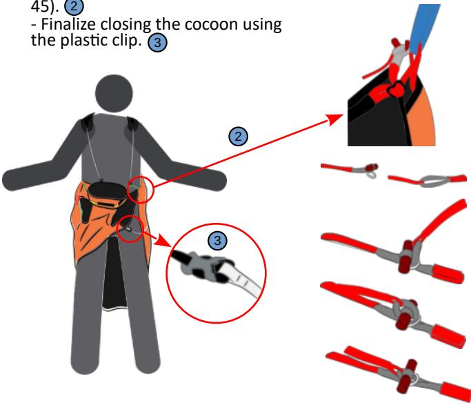
**Despite the presence of an anti-forget system, it is essential to pay particular attention during the attachment phase in the harness.**
