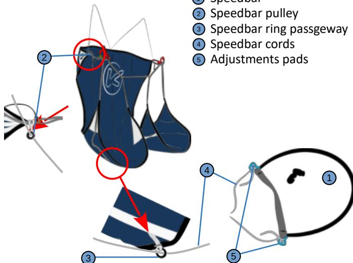
The speedbar adjustment is done at the level of the adjustment pads. Optimal adjustment allows you to take advantage of the entire speed range of the wing, when the second rung is pushed out with your legs stretched out.
