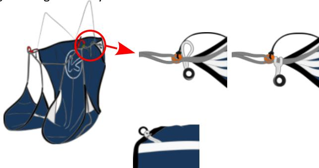
To install the optional speedbar, simply pass the cord through the pulley located on the side of the harness, then insert it into the ring located at the front of the thigh.
