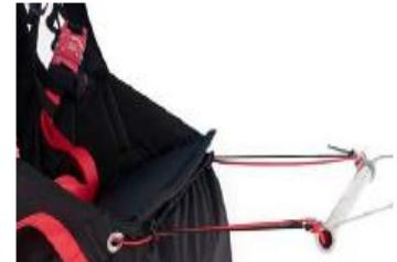
***Please pay attention that the glider will not be pre-accelerated, while the accelerator is loosened, when the acceleration ropes are set too short.***
