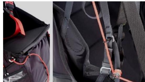
at the front right and left of the harness from the outside and then through the eyelets on the side.
