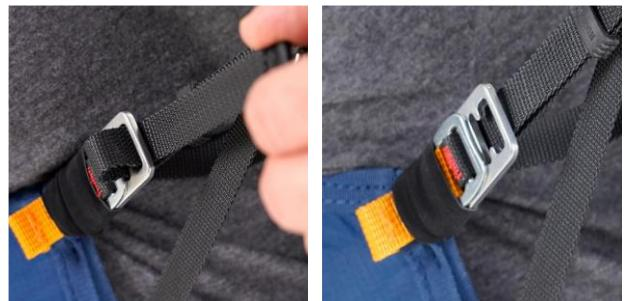
Our harness is supplied with the adjustment locked. To change the setting, you must first remove the strap from the lock, then you can adjust the inclination of the torso to make it more vertical by pulling the strap forward, or more reclined by pulling the light grey strap in the opposite direction.
