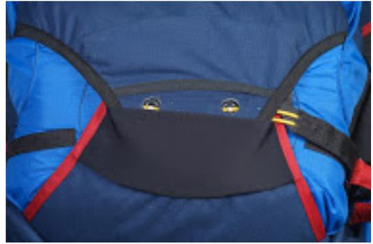
Position the handle in its folding sleeve.
