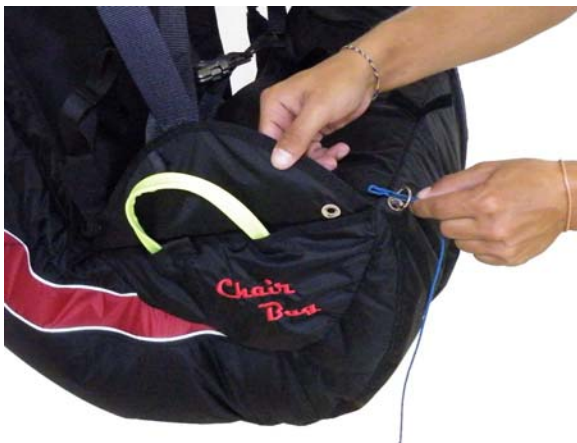
Brummel hook attachment to speedbar lines
