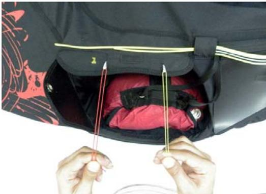
6. Take two short pieces of thin cord (i.e. glider line of approx. 40cm each, called "pull cords") and separately thread one through each of the white nylon closing loops attached to flap No.1 as shown.
