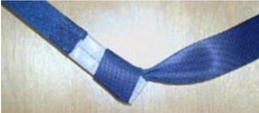
3. Attach the reserve parachute bridle to the center of the harness bridle using a larks head knot, sealed with a heat shrink tube to keep it in place as shown.
