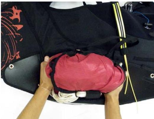
4. Place the deployment bag containing the reserve inside the reserve container of the harness, with the handle connection facing up as shown.
