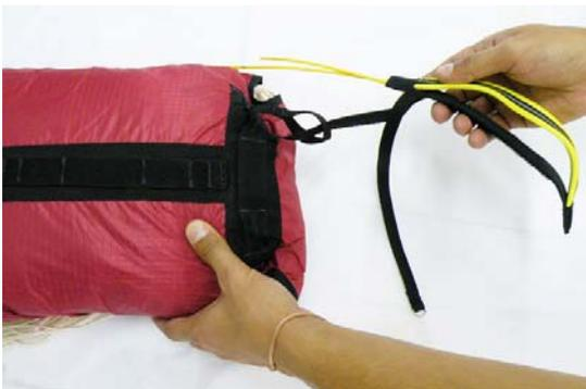
1. The handle has a split ring fixed to one of its attachment loops. Thread the first (without the Split Ring) attachment loop through one of the attachment points on the deployment bag. Pass the handle through the protruding loop to form a lark Head knot as shown.
