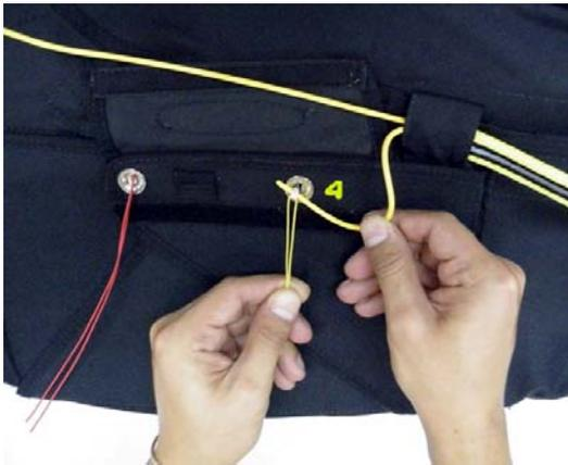
10. Next push the short locking cable through the first closing loop as shown, carefully remove the pull cords by passing one of its ends under the locking cable and pulling it out slowly.
