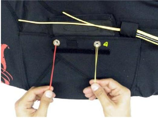
9. Next thread the both pull cord through the grommet on flap No.4.
