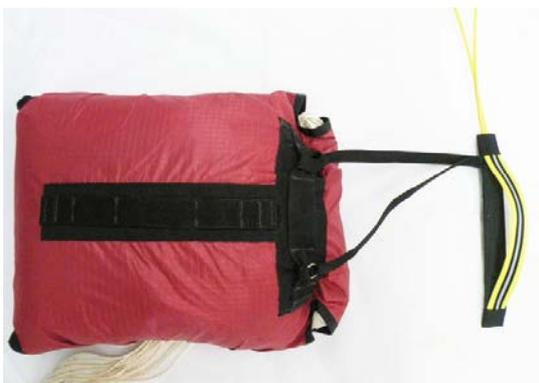
2. Thread the second attachment loop through the other attachment point on the deployment bag, making sure to center the split ring on the loop, passing it through first. Use the split ring to complete the second "larks head knot" by attaching it to both the strips of the attachment loop on the other side of the attachment point. The handle should now be attached at two points to the deployment bag as shown.
