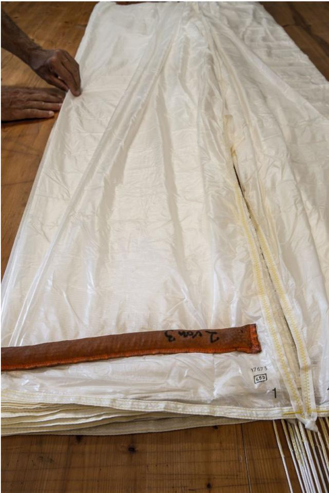
Panels with slots are laid out as cone.
