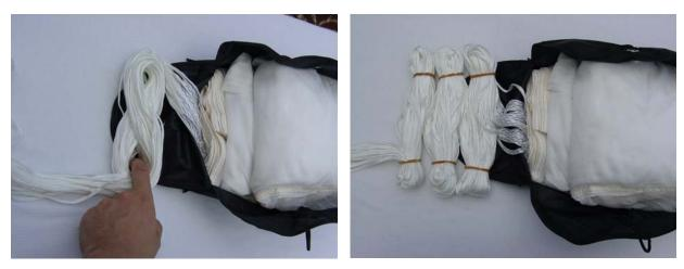
Put the canopy in a `S`shape into the parachute-opening-device (see picture 5). The lines will be placed with 3 by 3 aft on top of the closing-claps and secured with rubber band (see picture 6). These 3 line packages will be placed firmly near the parachute.
