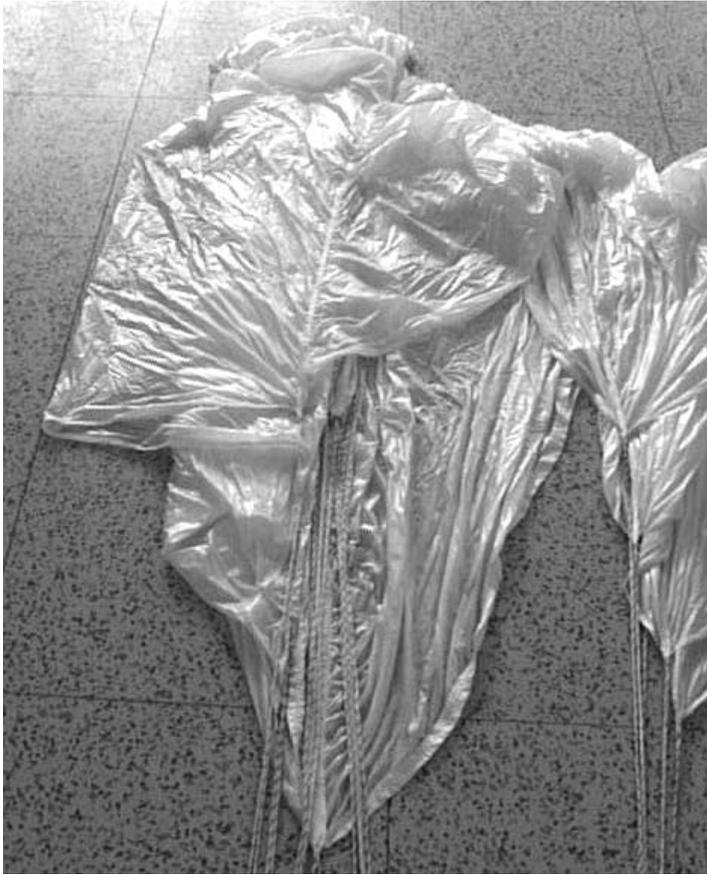
7) Again, folding of the next section is exactly the same. Make the folds so that individual support cord rows are next to each other and cords are tensed.
