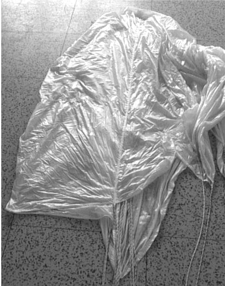
5) Layout the next section, fold the bottom edge of the section towards the parachute centre and then fold it in half towards the parachute centre.
