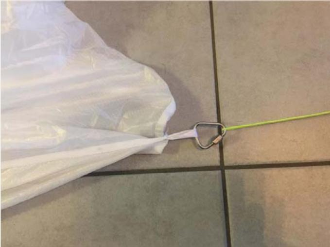
The Houston has only one packing loop. This is sufficient for easy packing of the canopy and saves time. The loop is aligned with the tension stripe on which the red front tip is also connected.
