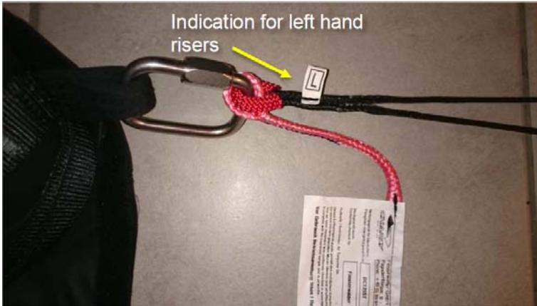
Install only approved connectors with at least 250 kg WLL (Work Limit Load). If you use Dyneema links, install them according to the instructions of the manufacturer. **Put both loops (riser and red safety connection) on each side into the shackle and tighten!** If your harness has an included V-line, remove it. **Do not connect the reserve parachute onto the V-line!**
