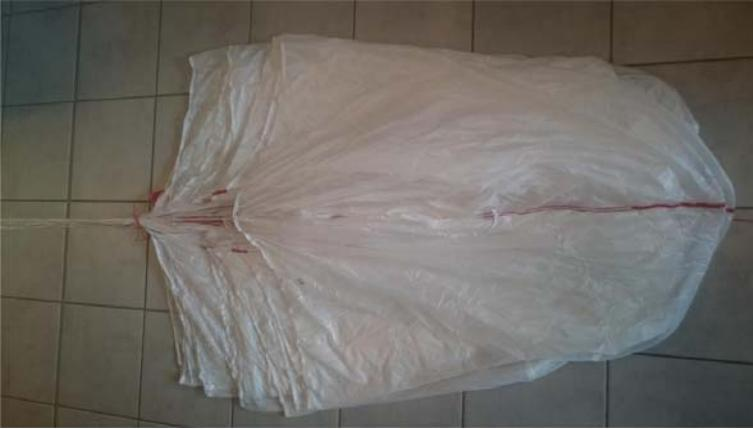
Fold-back half of the panels to the other side and remove the marking.
