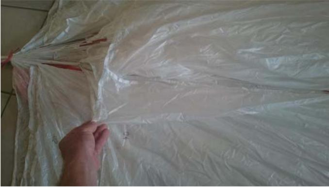
On the side tips, the stabilo triangles are located. No special fold is required for this part. Continue until the rear gap will appear.
