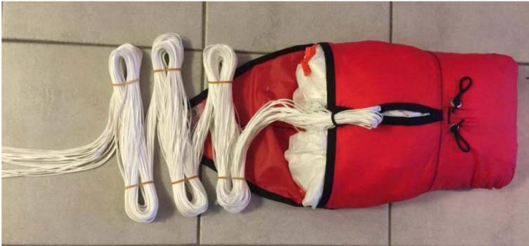
Position the lines according the picture and bundle the lines with three loops (max. 4 loops) on each side of the bundle.
