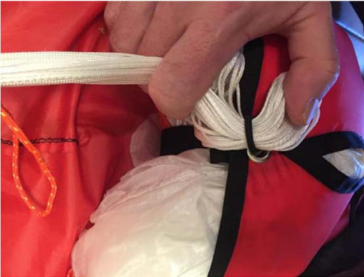
Take the rubber loop and both leaves of the container and close it with the bundle of lines. Only lead the rubber loop through the two lugs.
