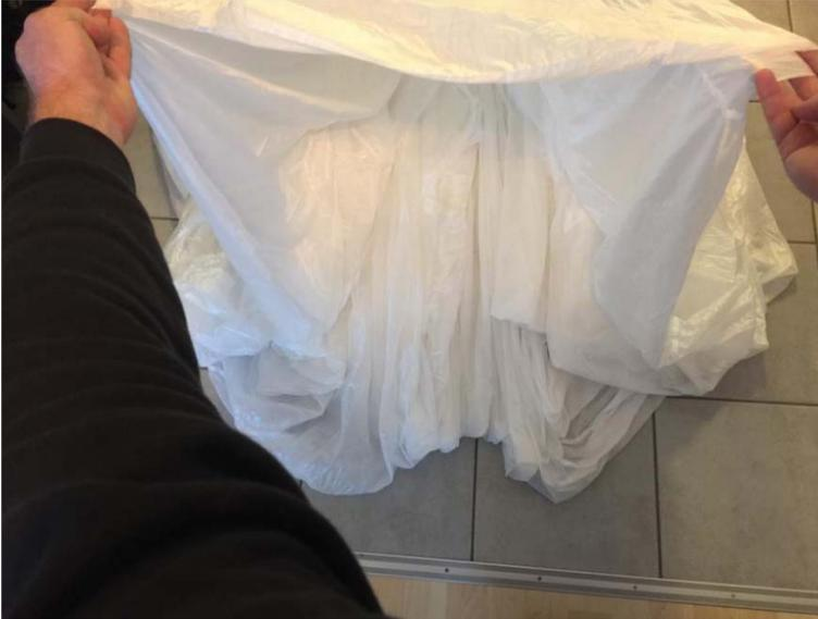
Pull back the material of the canopy around the contour of the parachute, so that the main, center, and brake lines are pre tensioned. This makes folding of the canopy easier.
