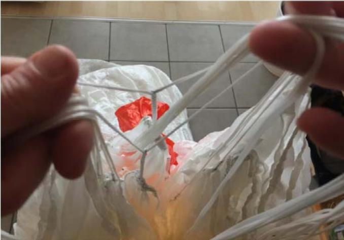
Continue to the canopy and check that all centerlines are between the two front and two rear fork lines. **CAUTION: If the center lines are not between, there is a line over and the canopy is inside out!**
