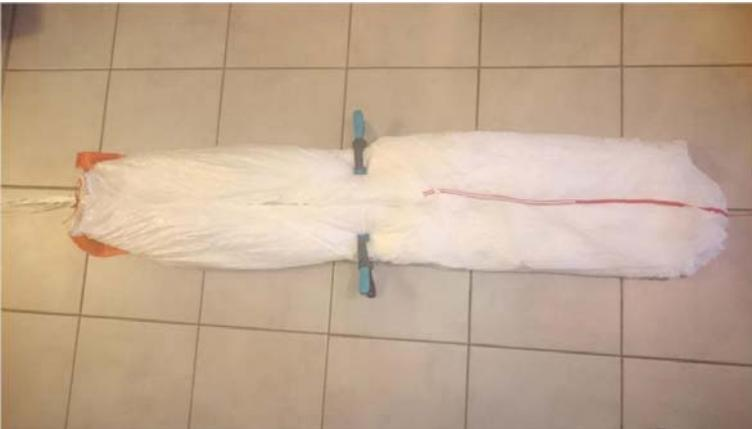
Align the rear tip over the panels, open the rear gap and hold it in position with the clamps.
