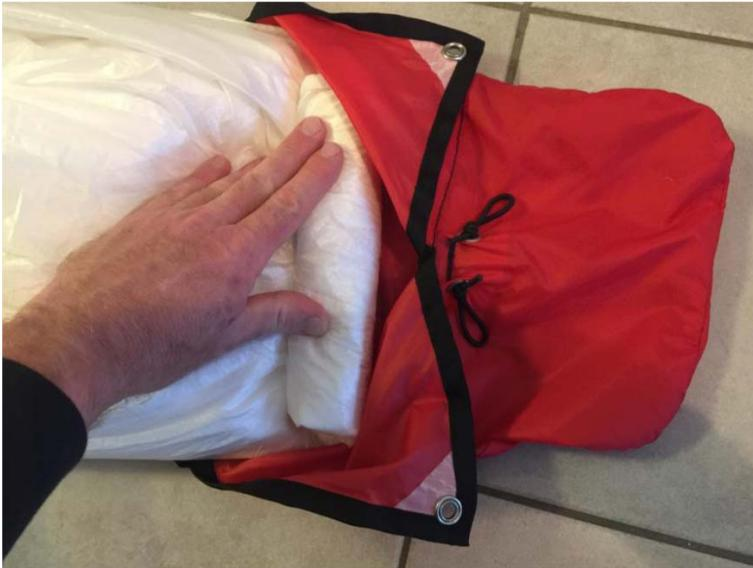
Wind-up approx. 10 - 15 cm of the top of the canopy and put it into the bottom of the inside container.
