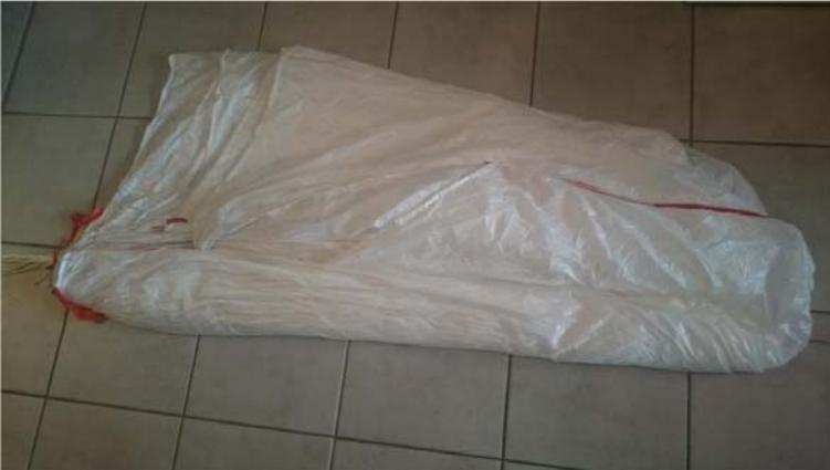
Fold panels two times at approx. 1/3 of depth in direction of the center (no S-folding!). Do not fold too narrow as the height of the container will increase. You may use packing clamps or weights.
