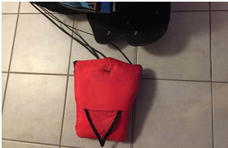
Move harness into upright position, install handle on the inside container. Pack risers (like V-lines) and container into the harness according the instruction of the harness manufacturer.
