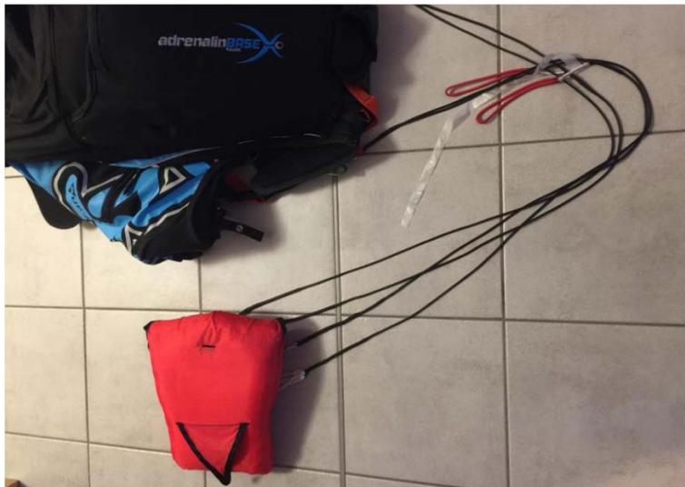
Move the container in the twisted position to the right side of the harness, if the container opens on the right side. Otherwise move to the opposite direction.
