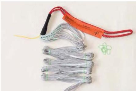
The lines are collected in S-folds so that it gives about 3 - 4 line bundles. Again, care should be taken that the excess of the line loops behind the rubber are kept as small as possible.
