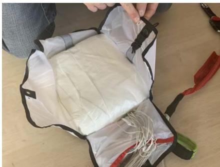
The leaves 1 - 4 of the inner container will be closed with the black rubber line loop in the correct order.
