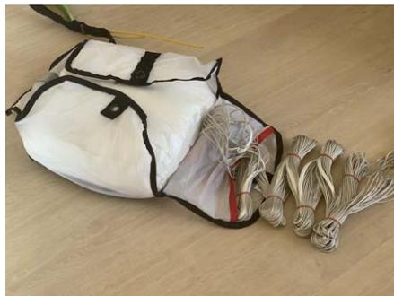
The lines are collected in S-folds so that it gives about 2 - 3 line bundles. Again, care should be taken that the excess of the line loops behind the rubber are kept as small as possible. From the last line groups to the main riser should be left 40 cm of lines for closing the cover part.
