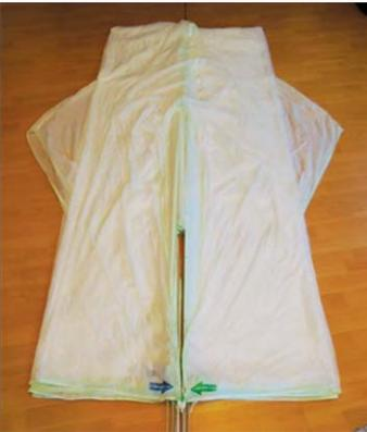
The other panels are placed clean down till the top corner panel is achieved. This panel is recognizable by the two arrows pointing to each other. The Aegis SQ is now symmetrical and nicely folded in front of you.
