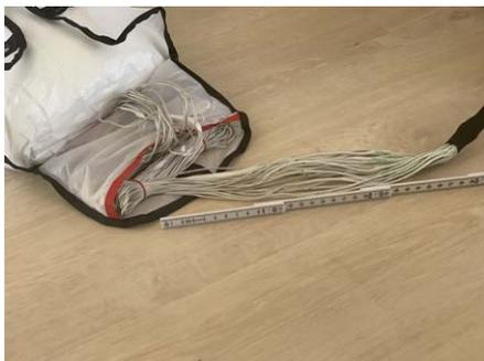
The line bundles are stowed in the pocket of the line bag of the inner container.
