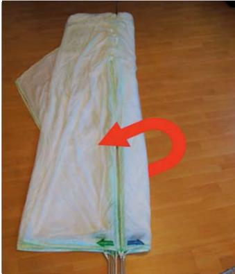
The entire parachute is now rotated around its axis 180° to the left. This act is the most difficult and it is easier if two people working in sync for the rotation. At the base edge the two arrows pointing away from each other are now visible.
