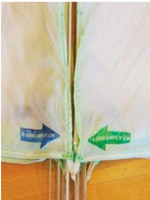
The base can be seen below with the centrally located lines, all panels with the blue arrows are left and all panels with green arrows are the right of the lines. In the middle are the arrows which are pointing to each other.
