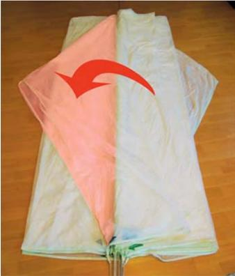
The fourth panel is a blue corner panel as already on the right side and is accordingly also laid down as flat as possible.
