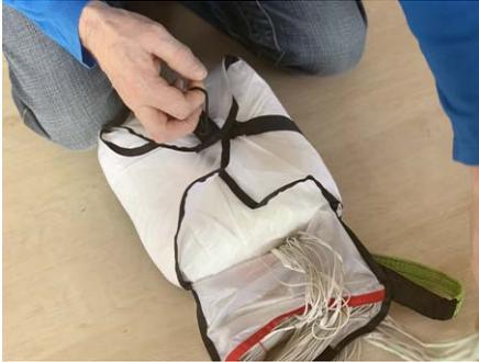
Lead the black rubber loop through the grommet of the leaf no. 3.
