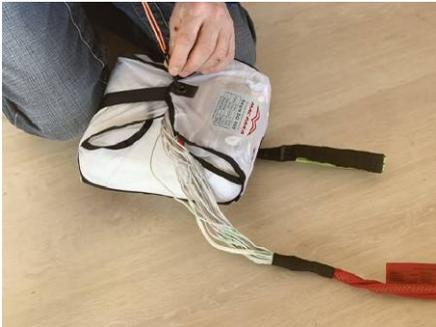
Then lead the black rubber loop through the grommet of the leaf no. 4.
