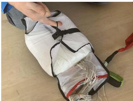
Lead the black rubber loop through the grommet of the leaf no. 2.
