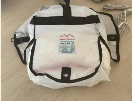
The inner container is placed on top of the existing S-turns. The slot of the inner container should look towards the lines.
