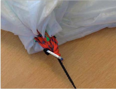
Before each packing slide on the packing loops on a line (packing cord). Now you pull the whole rescue under tension, all the fabric and lines are under tension except the 4 corner lines.
