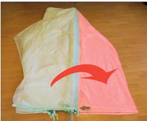
Now you have to arrange panel by panel to the right (green arrows). The panels should be as wrinkle-free as possible. Note that the lines remain pooled on the basis below. The first panel has come to be tapered at the top.
