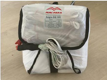
Use the remaining free line to secure the black rubber loop of the inner container.
