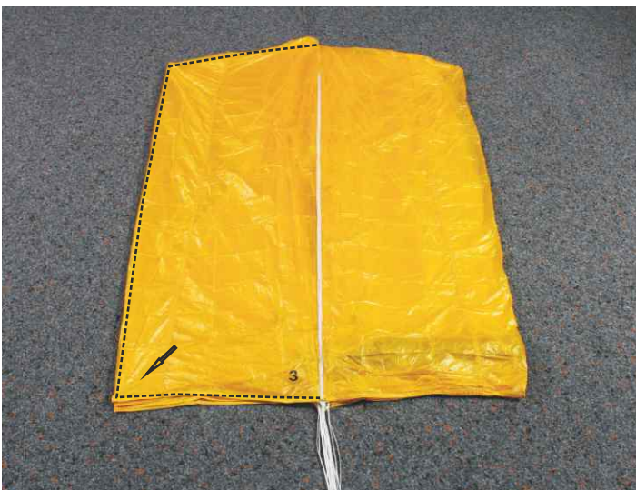
17. Arrange panel 3 (Ultra Cross 100/125). Ultra Cross 150: panels 4+3
