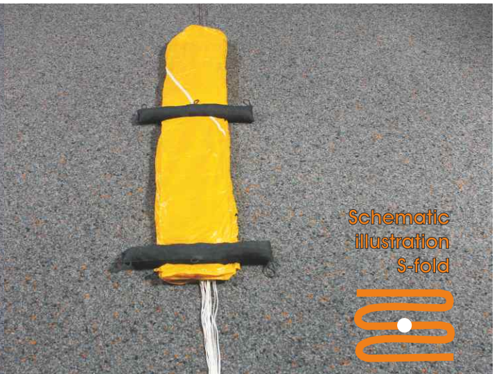
22. Fold left side S-shaped (Step 2).
