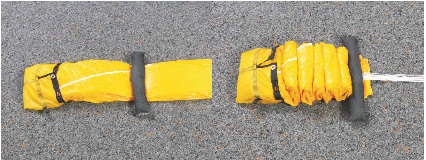
24. Stow top of the canopy in the deployment bag.
