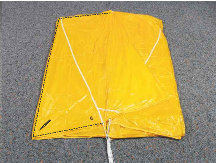
14. Arrange panel 6 (Ultra Cross 100/125). Ultra Cross 150: panels 8,7
