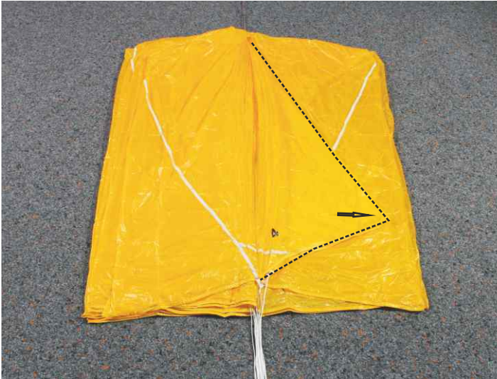
7. Arrange panel 4 (Ultra Cross 100/125). Ultra Cross 150: panel 5
