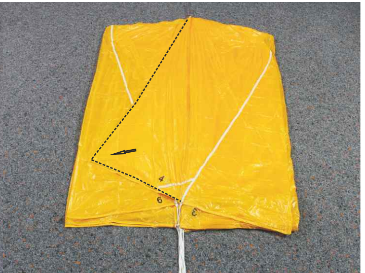
16. Arrange panel 4 (Ultra Cross 100/125). Ultra Cross 150: panel 5
