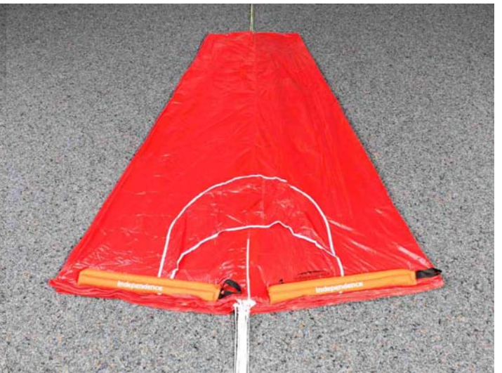
6. When all segments are laid properly put a weight (sand bag) on both sides.
