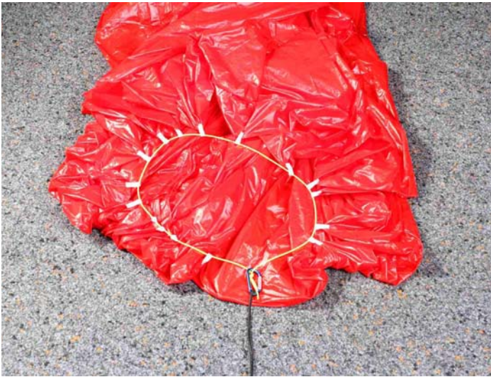
1. Slide on the packing-loops on a line (packing-cord), and hook it in.
