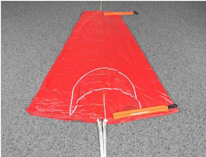
3. Lay all segments until segment 1 (stamped segment) is on the top, then put a weight (sand bag) on it.
