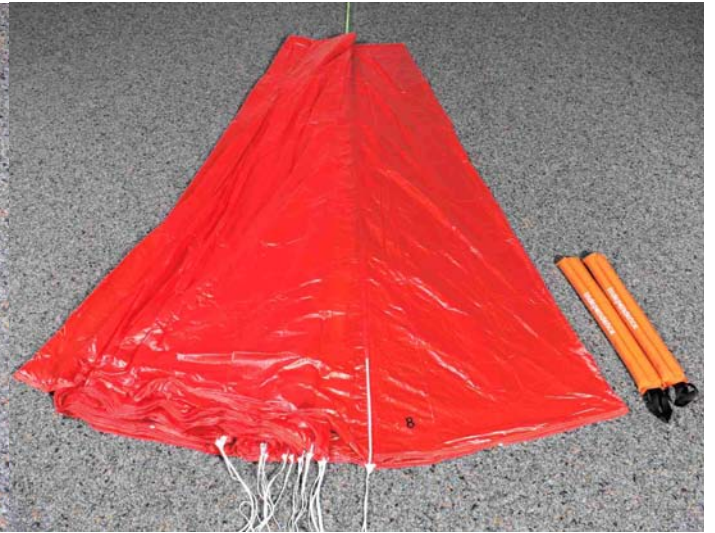
2. Segment 8 have to be put on the right side.
