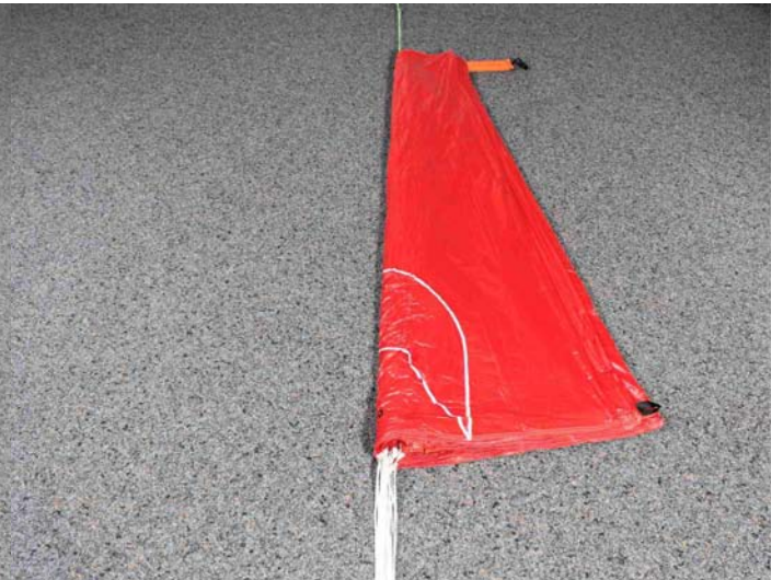
4. Fold the left side onto the right side.
