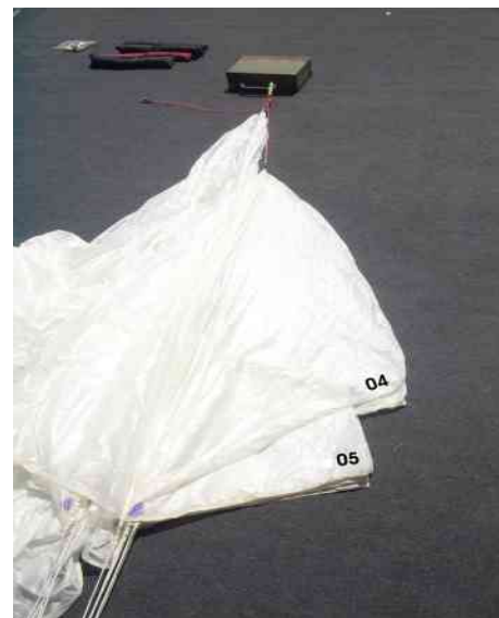
8. Attach apex of the third and last canopy, and put the between-segment No.04 on segment No.05.
