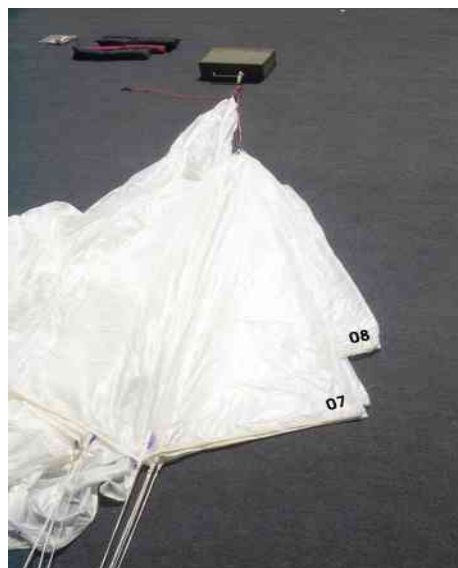
7. Put segment No.07 on segment No.08, No.06 on No.07, and No.05 on No.06.
