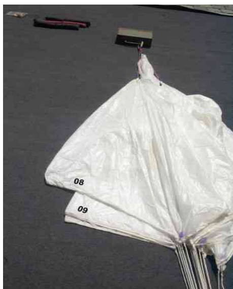
11. Put the left segments, according to point 3-6, on the left side now.
