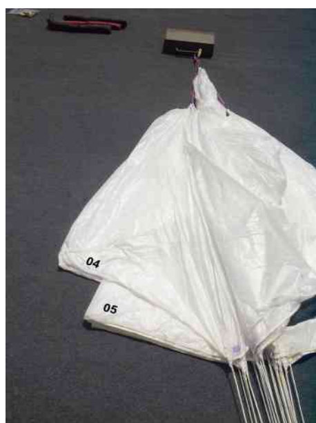
13. Attach the apex of the third and last canopy and put between-segment No.04 on segment No.05.
