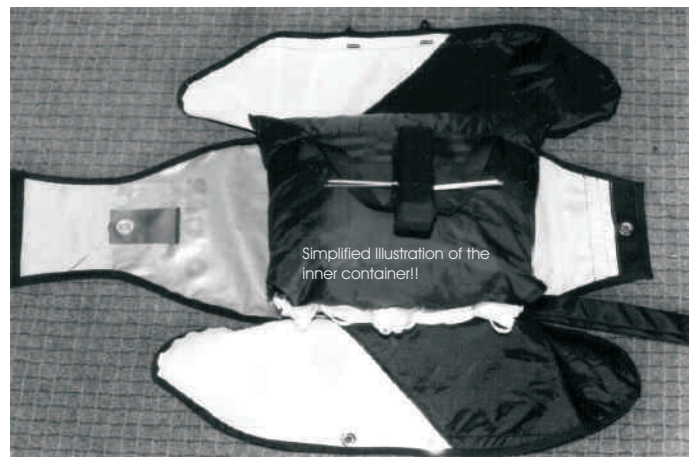
26. Arrange the bridle on the left or right side, depending on the needs of the pilot.
