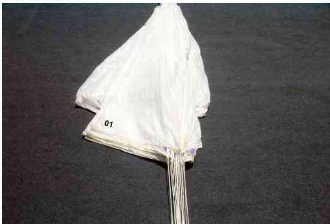
17. Fold the canopy in form of a "S". Approximate 1/3 of the right side is put under the lines.
