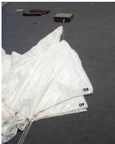
6. Attach the apex of the next canopy and put the between-segment No.08 on segment No.09
