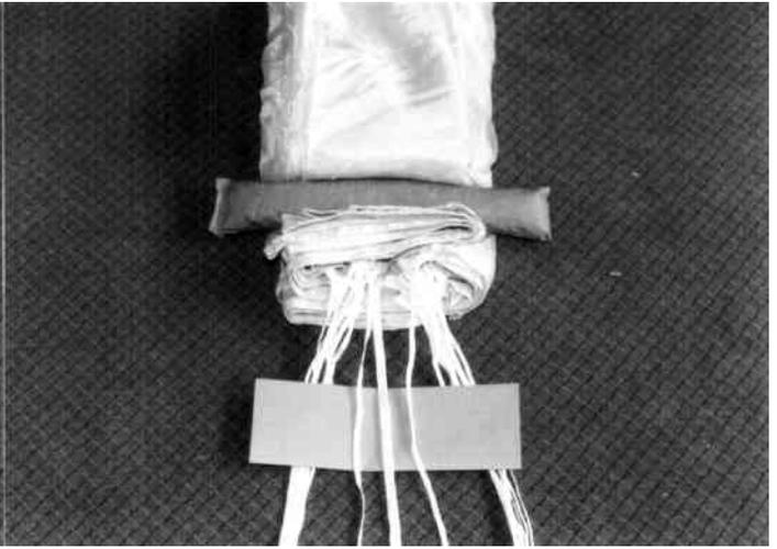
6. Inspect the lines 1 and 20 and the center lines. Check that none of the lines are twisted.
