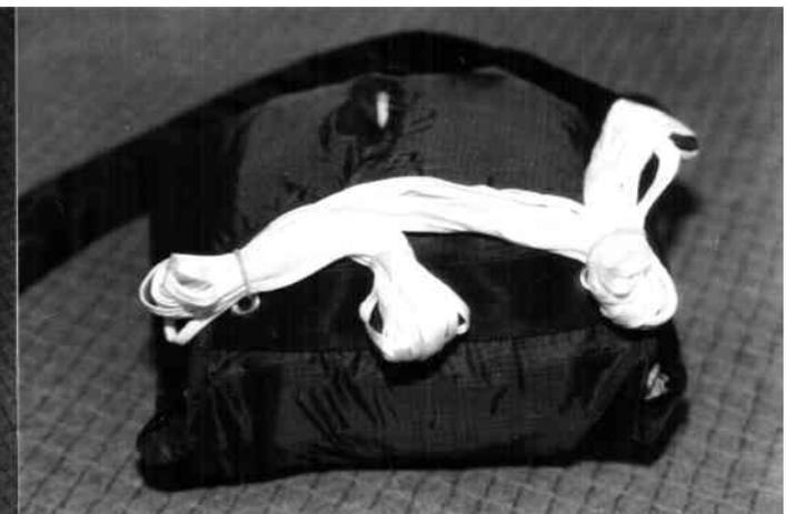
10. Close the inner container with the last 50 cm of lines. Start with the middle, finish with the outer.
