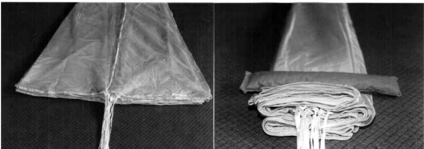
3. The canopy is placed on the table and folded such that the stamped segment (No. 1) lies on the top. The same number of segments are now on the left and right side.
