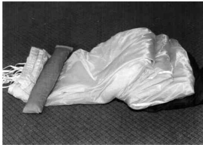
7. Place the parachute in the container in the form of an "S". At first make 3 "S" folds on the inner container. Leave the last 40 cm without an "S".
