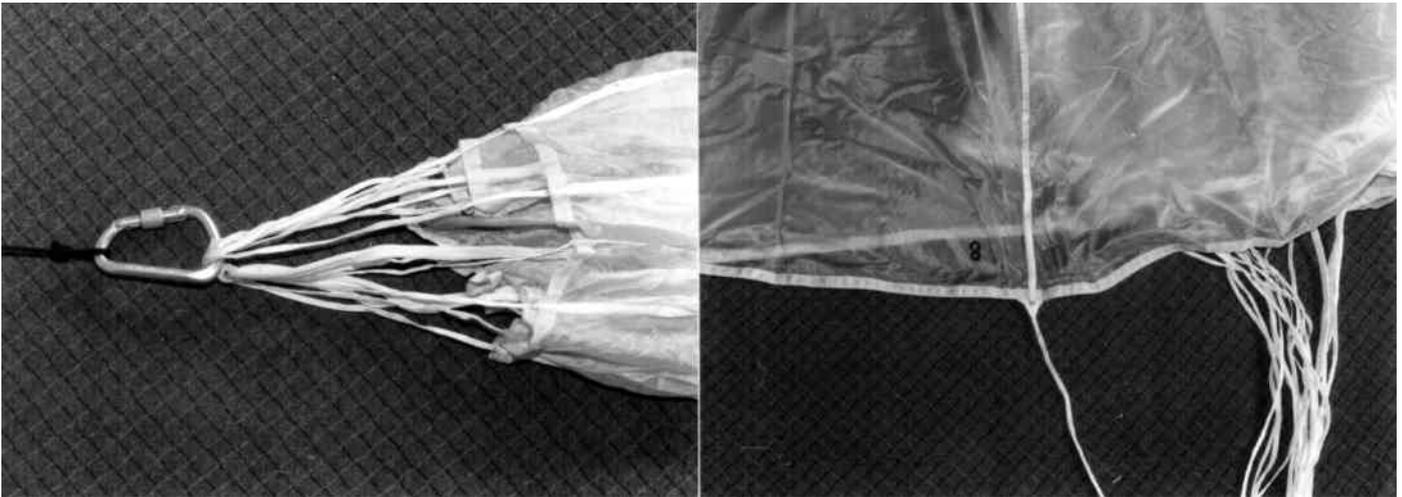
1. Secure the parachute at its apex to a suitable hook.
