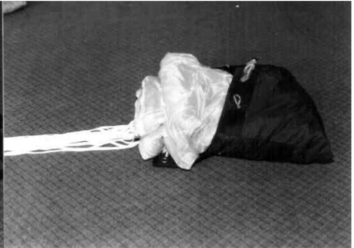
8. Take all "S" folds and put it inside of the inner container. Fold the last 40 cm in small "S" folds in the inner container.
