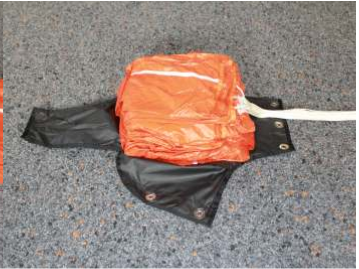
28 b. Fold the rest of the canopy in S-folds (stack-pack).
