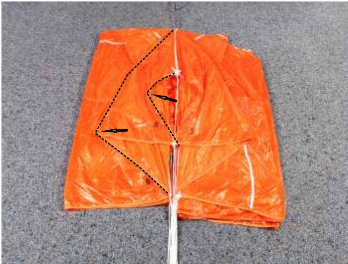
19. Arrange panel 5 (corner panel) (Evo Cross 160:panel 6)
