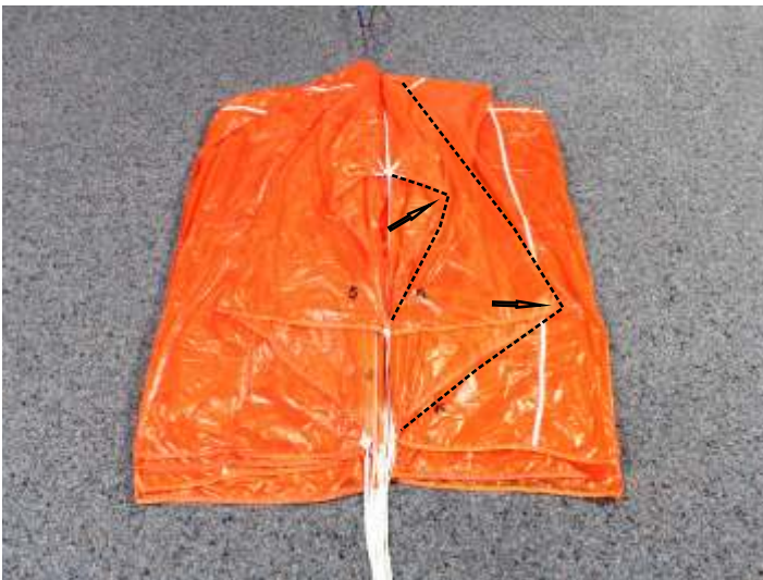
9. Arrange panel 5 (corner panel) (Evo Cross 160: panel 6)
