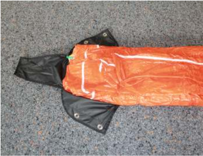
27 b. Stow top of the canopy in the deployment bag.
