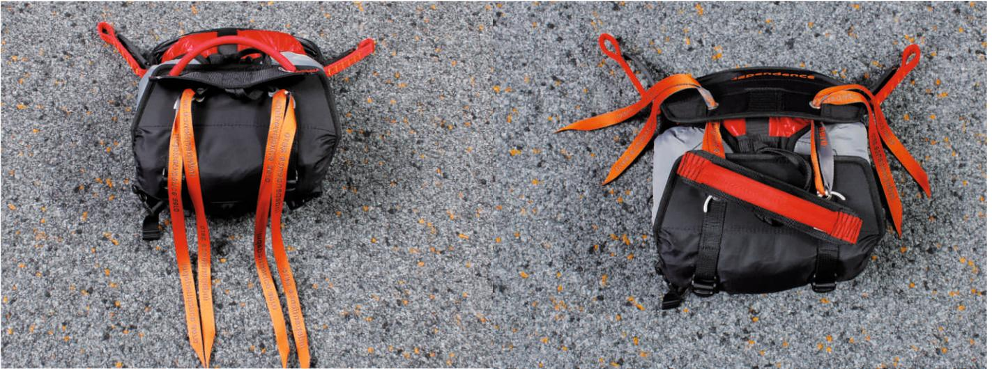
6. Close the bottom flap and secure provisionally with the pins of the release handle.
