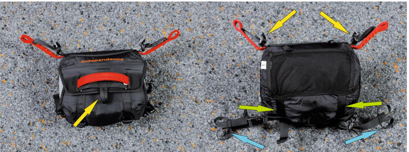
8. Close the top flap and secure with the pins of the release handle. Stick the release handle under the handle cover and remove packing cords. Take care that the handle - deployment bag connection (arrow) is long enough that the pins will unlock the flaps.
