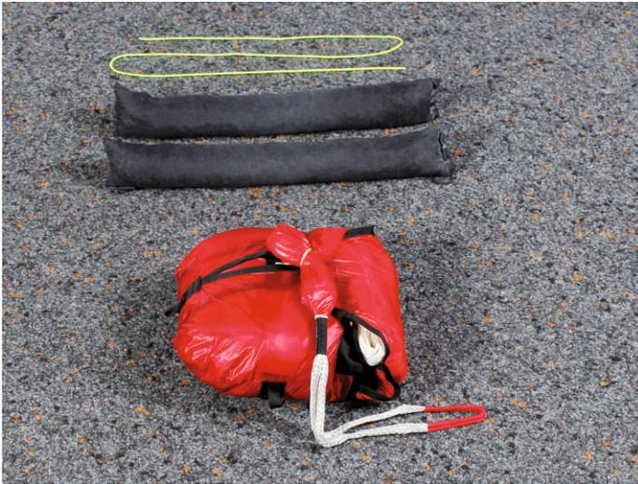
23. Close the lines deployment bag with the last 60 cm of lines.
