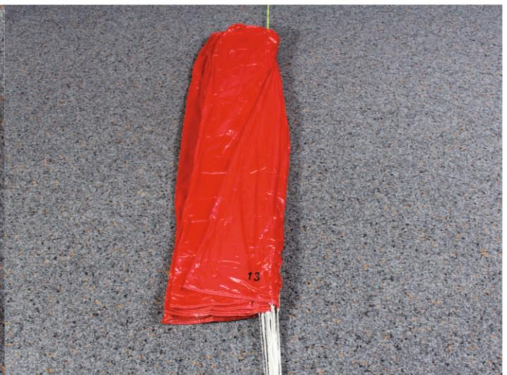
1. Slide on the packing loops on a packing cord. The number and placement of the packing loops can be seen by 15.1.
