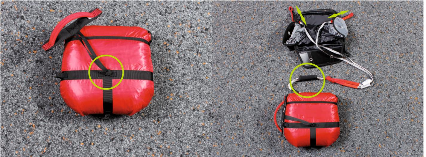
1. Connect the release handle at the loop in the middle of the deployment bag (flat side) by looping.
