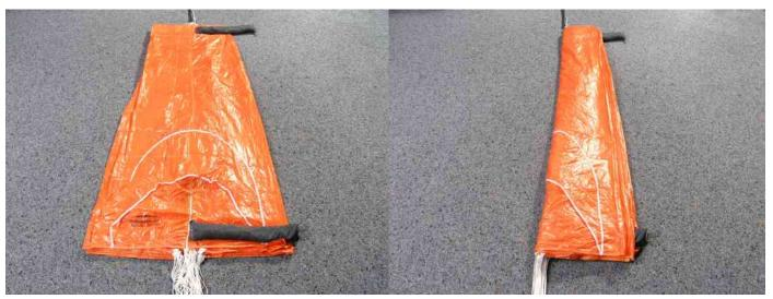
3. Lay all segments until segment 1 (stamped segment) is 4. Fold the left side onto the right side. on the top, then put a weight (sand bag) on it.
