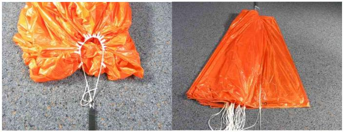
1. Slide on the packing-loops on a line (packing-cord), and hook it in.
