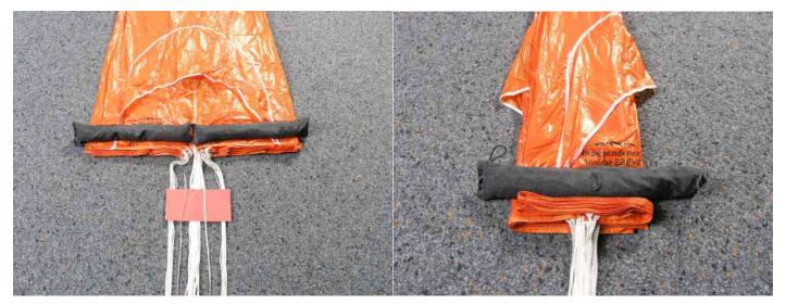
7. Check that line 1 and 20 (Annular Classic 20) and the center line are not crossed and running free. (Annular Classic 22/22HG: 1 and 22; Annular Classic 24/24HG: 1 and 24; Annular Classic Tandem/ Tandem HG: 1 and 30; Annular Classic 36 Tandem/36 Tandem HG: 1 and 36)
