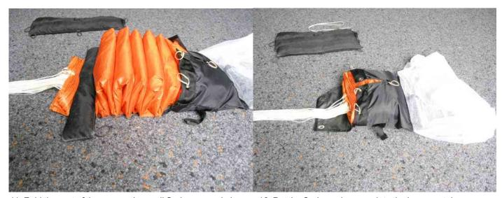
11. Fold the rest of the canopy in small S-shapes and place it in front of the innercontainer.
