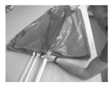
Place the data sheet gore on the right side of the table. Grab the first two suspension lines together with central line and start flaking each wedge out with the other hand, adding subsequent lines to the bundle. Stop after flaking half of the total gores number.
