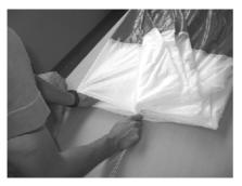
In the end check that no wedge was overlooked and there is the same number of wedges on each side. Sort the top part of the canopy.
