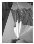
Find the first outer suspension line and keeping it in hand go to a data sheet gore. Further along this line there are assistance straps sewn into top part of the canopy. Lead an assistance line through these loops and fix it to the other edge of the table.
