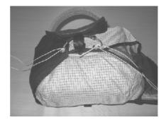
Close the container side lids using assistance lines and pins.
