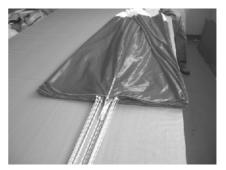
Gores and wedges have to be pulled out completely and accurately. After completing right half of the canopy, cover it with the unsorted left half and start over again.
