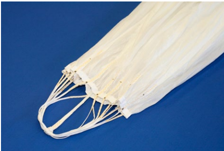
1.1. Inspect the middle apex for symmetry
