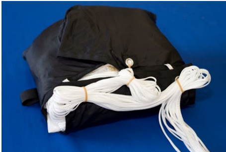
3.5. Lay the 3 x 8 bundles of suspension lines on the canopy in the inner container, and fasten the container lid from the middle to the outside using the remaining suspension lines.
