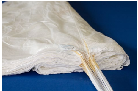
2.6. Now the complete bundle of suspension lines together with the left hand panels must be carried back over to the middle of the first laid panel.
