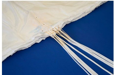
1.4. The bridle line is fixed to the lower end of the packing table and the reserve is stretched. The suspension lines are checked to ensure that their course is straight.
