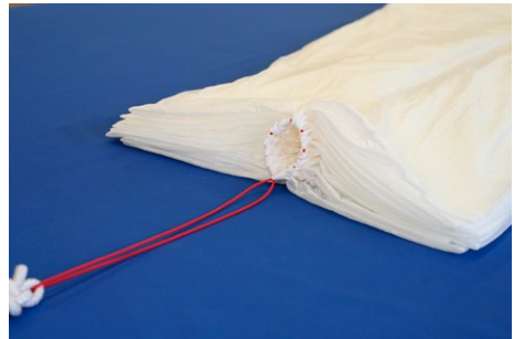
1.2. Pull a draw cord through the packing loops and attach to the upper end of the packing table:
