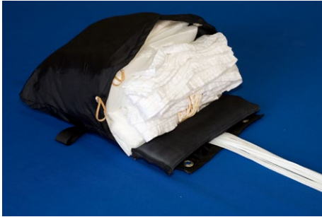
3.3. Lay the s-shaped canopy in the inner container and use a packing weight to prevent the canopy from sliding out.
