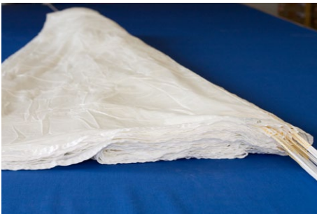
2.5. In order to lay the canopy in S-shapes, the complete bundle of suspension lines and the left hand panels must be lifted slightly and laid 2/3 over the right hand panels.
