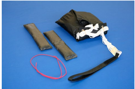
3.6. Check that all packing tools / aids / draw cords that were used, have really been removed.
