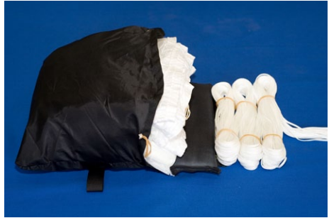
3.4. The suspension lines are now placed in figure eights and held in place using the new special rubber bands. Pay attention that the width of the inner container is not exceeded. The last 50cm of the suspension lines are used to close the container and must remain free from rubber bands.
