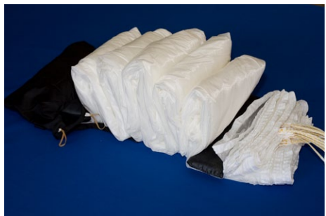
3.2. Sort the rest of the canopy into small S-shapes in front of the inner container.
