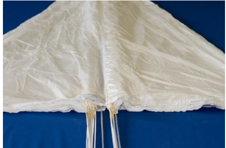
2.4. Before laying out the suspension lines in an S-shape, ensure once again that all lines are untangled and do not cross over one another.
